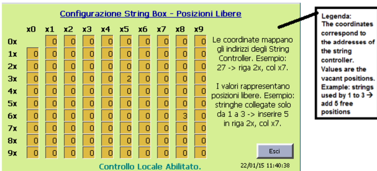
Fig. 21. Example of screen “String Box configuration – Free Position”.
