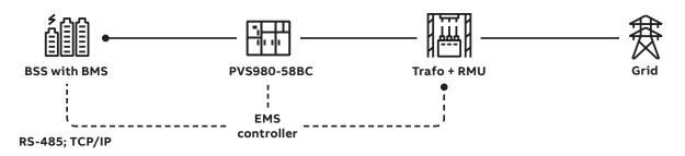
ABB's new high-power energy storage power conversion system is ideal for multi-megawatt energy storage plants. It features high voltage DC for system cost savings, a self-contained cooling system, fast responding controls and is designed for harsh environmental conditions.
