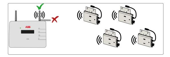
When configuring the CDD and acquiring the inverters in part 4 and 5, it may be necessary to adjust the positioning of the antenna. The RF signal quality is shown in the CDD display (see part 3).
