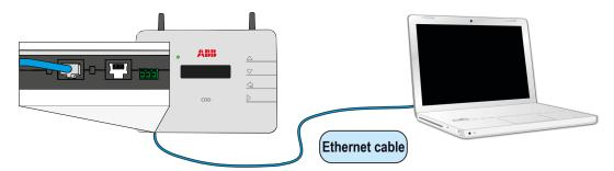
If the computer is directly connected to the CDD without a router, and if the computer is set for an automatic IP address, it is necessary to change the Network settings on the computer following the procedure below:
