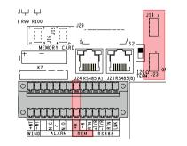
PVI-10.0/12.5-TL-OUTD (Construction A) Cable to be used: Model 1 Adapter board: Yes
