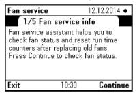
3. Change between different fans (Internal fan, External fan 1, External fan 2) menus with **Back** and **Continue**.
