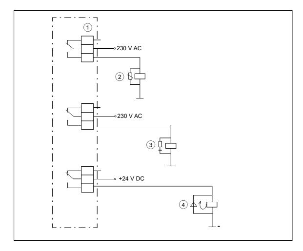
1) Relay outputs, 2) varistor, 3) RC filter, 4) diode
