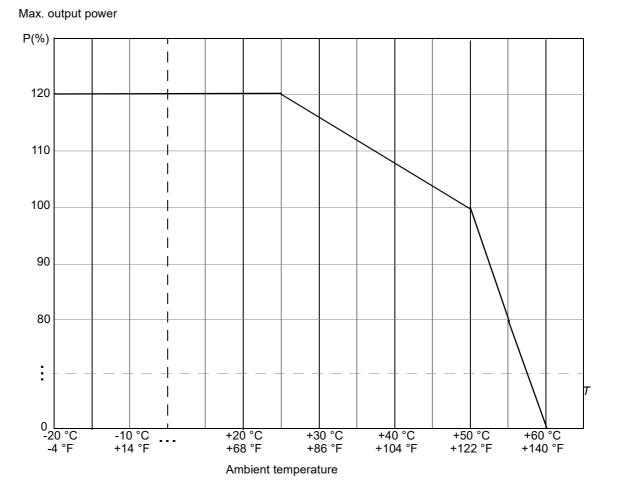
Use the following correction factors when you calculate the available inverter power at different temperatures:
