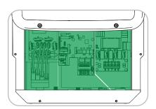
• Disconnect the grid voltage (by switching off the protective device upstream of the inverter).
