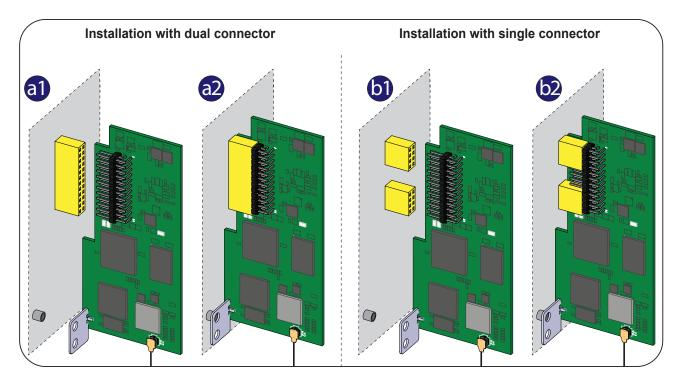
During this stage, **carefully** check that all the terminals are correctly aligned. Any misalignment of the terminals may result in irreversible damage to the board and/or inverter!
