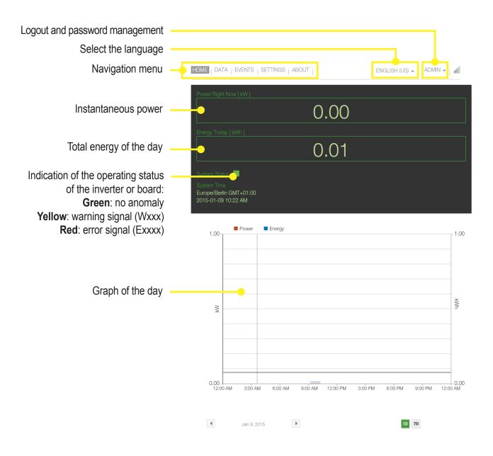
The DATA page displays a summary of the most significant technical data for the Wi-Fi board and the inverter. The real-time data is updated every minute, while the system information gathers the main characteristics of the installed devices in a table.
