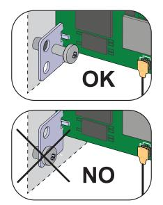
Tighten the locking screw to secure the board to the inverter. This screw secures the mounting bracket to a specific anchor point on the inverter and prevents any unintentional disconnection of the board.
