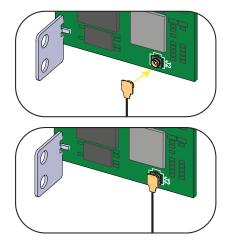
Before installing the board inside the inverter, connect the antenna cable to the coaxial connector on the board.
