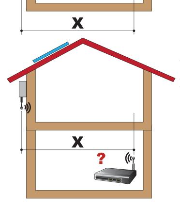
**Distance X between the Inverter and the Wi-Fi Router:** greater than 10m/33ft and/or with obstacles or floors to pass through.
