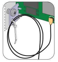
The second hole on the bracket can be used to secure any excess antenna connection cable, using the strap supplied.
