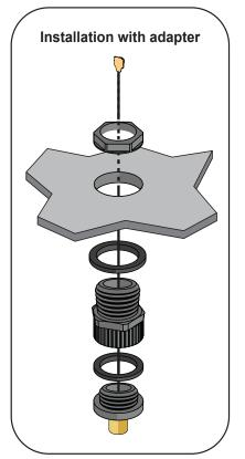
For installations in inverters for which **the adapter is required**, proceed as follows:
