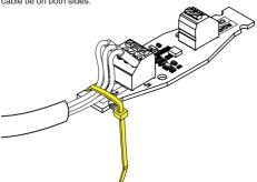
After the cable fixing, close the enclosure (04) to complete the DRM0-INTERFACE assembly.
