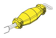
After the assembly, make sure to put the DRM0-INTERFACE inside the inverter enclosure in a suitable position: The DRM0-INTERFACE device position cannot interfere with mobile parts of the inverter (fans, switch...) or dangerous electrical parts.
