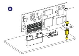
After the installation of the adapter board to the inverter it will be possible to connect the DRM0-INTERFACE to the adapter board using the specific connector of cable "Model 1" as shown in the picture (C).
