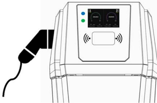
8. When the battery of the electric vehicle is fully charged, the LED will turn steady GREEN
