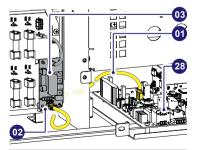
NOTE – the wiring must be passed through the bottom of the partition (DC side / AC side of the wiring box) together with the other cables present on the wiring box. • Connect the wiring negative pole (05) (wiring code ZLH.V3R05):
