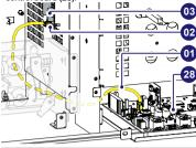
NOTE – The wiring must be passed through the bottom of the partition (DC side / AC side of the wiring box) together with the other cables present on the wiring box
