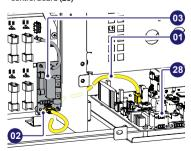
NOTE – the wiring must be passed through the bottom of the partition (DC side / AC side of the wiring box) together with the other cables present on the wiring box.
