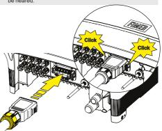
• Secure the AC quick fit connector. Install and screw the holding clip.
