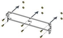
· Attach the bracket (05) to the support.
