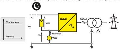
Array terminal voltages with respect to ground during night-time PID recovery operation (inverter is off-line).
