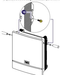
• A padlock can be installed to lock the inverter to the bracket so that it cannot be disassembled by outsiders.
