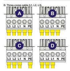
· Install ferrule with plastic collar on the wires.
