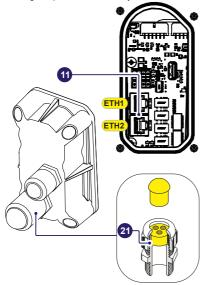
⚠ ATTENTION – If the inverters need to be connected in daisy chain or ring configuration use both connectors.
