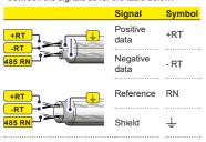
⚠ ATTENTION – Use a shielded twisted pair cable with characteristic impedance of Z0=120 Ohm in case of long distance connection.
