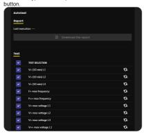
NOTE – While one of the tests is being performed, the set limits will be gradually increased/reduced (depending on the type of test) until the threshold at which the inverter is disconnected from the grid is reached. The procedures for running the Autotest comply with the legislation in force.
