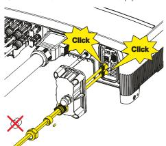
Install the signals connection box (08) by screwing the 4 locking screws present on it (see paragraph "3.5.2 Tightening torques").
