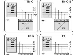
NOTE – The connection of the neutral (N) on the inverter is optional (dashed line on the above schematics); the inverter will automatically detect the presence or absence of the connection without any setting by the user.
