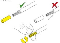
• Crimp the terminal to the conductor using the designated pliers.
