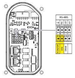
READ THE MANUAL – The external switch used for Remote ON/OFF should be rated for DC low voltage, low current application (the minimum switching current capability should be 1mA or lower).
