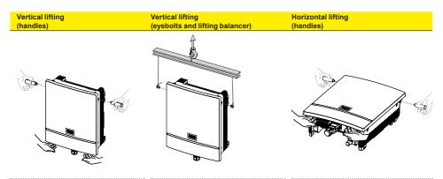
⚠ ATTENTION – DO NOT grab the equipment from the rear flange! Risk of injury due to cutting surfaces and risk of equipment damage. Always use proper lifting equipment!
