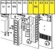
•Connect the wires according to the following table. The input that is "Closed" must be short circuited with the "K RN" terminal.
