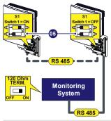
NOTE – The communication line must also be terminated on the first element of the chain which normally corresponds to the "third party system".
