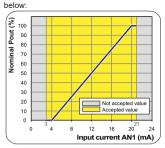
The reactive power limitation manages the output active power according to the current (4...20 mA) signal.
