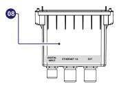
PVS-20/30/33-CCB must be connected to inverter USB connector (10) located under the Signals connection box (08).
