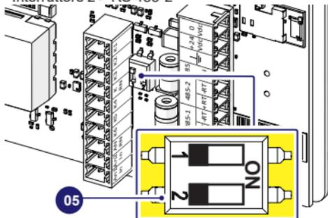
**NOTA** – Activate the termination resistance on the final unit of the chain.
