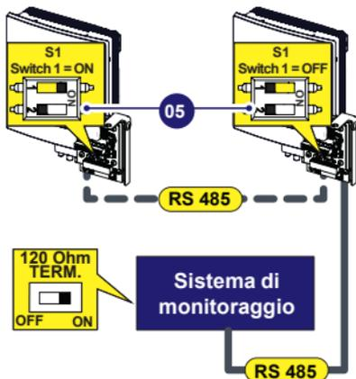
**NOTA** – The communication line must also be terminated on the first element of the chain which normally corresponds to the "third party system".
