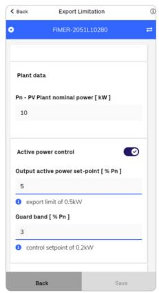
The guard band is the control margin used to achieve the export limit and is expressed as a percentage of the PV plant nominal power.
