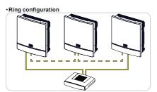
MOTE - In case inverters are connected to the networking switch with a ring topology is recommended to enable SPT protocol on the switch (Spanning Tree Protocol SPT (IEEE 802.1D) is enabled by default on inverters.
