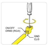
•Connect the wired screw terminal block to the Digital Input connector (12).
