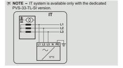
To connect the inverter to the grid could be use a connection cable:
