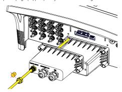
Install the 2 poles screw terminal block (supplied) on the cable (see paragraph "3.5.3 Tightening torques").
