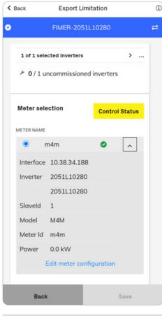
⚠ ATTENTION – Meter must be configured with generator reference system. Use the edit configuration link and follow the procedure in the next step to manage the link reference system.
