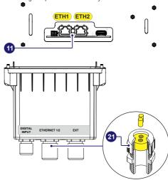
${\textstyle\bigwedge}$  ATTENTION – If the inverters need to be connected in daisy chain or ring configuration use both connectors.
