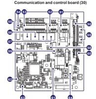
READ THE MANUAL — See the manual for details on the connections and functions available on the communication and control board. The illustration shows the main components and connections available on the communication and control board (30). Each connection cable reaches the communication board through service cable glands (13) and Ethernet cable gland (12).
