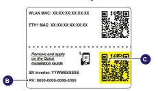
The inverter has an embedded Wi-Fi module that creates a wireless network named FIMER-YYWWSSSSS, where YYWWSSSSS is the serial number (SN) found on the Communication Identification Label. For example, FIMER-202401000001.
