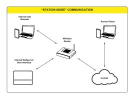
NOTE - Where possible, connecting the inverter in "Station Mode" is always preferable. Thanks to the internet connection, this mode ensures better operation.
