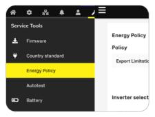
MOTE – If a meter is installed, after completing the wizard, access the WEB User Interface as ADMIN (default password is 0010) to configure the chosen policy. The available options are Self-consumption or Export-limitation. You can download the "Power platform Energy Policy overview" application note from the FIMER website.
