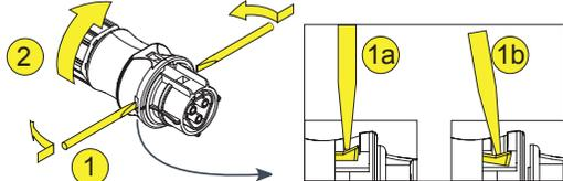
• Insert the cable into the connector and cut the cable to length
