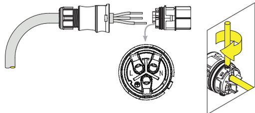
• Close the connector and tighten the cable gland respecting the tightening torque (4+1 Nm) to ensure the IP65 degree of protection
