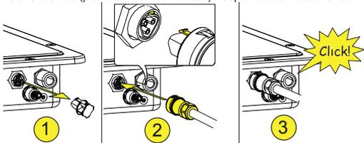
**⚠ ATTENTION –** To maintain the IP protection rating of the inverter, it is mandatory to install the counterpart with the AC cable connected or the protective cap, on the AC output connector. In addition, the connector must not be subjected to tensile forces (examples: do not connect weights to the AC cable, do not leave excess wire hanging, etc.).
