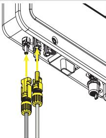
**⚠ ATTENTION –** The use of non-compliant counterparts with respect to the quick-coupling connectors models present on the inverter, may cause serious damage to the unit and result in the immediate loss of warranty
