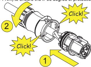
• Remove the pre-installed protective cap on the inverter. Insert the counterpart in the AC output connector (10) while taking care to align the references (present in both connectors) that prevent connection errors.
