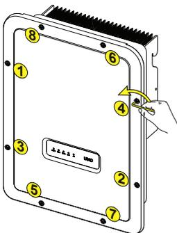
After making the connections, close the cover by tightening the 8 screws on the front, while respecting the sequence and tightening torque (2.5 Nm).
