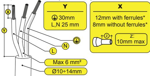
(\*): Use properly crimped ferrules only on stranded wire with a conductor section values between 1.5 - 4 mm<sup>2</sup>.
