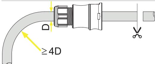
• Prepare the cable according to the following measurement:
