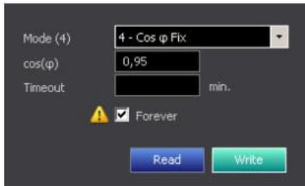
Figure 32: SA12 Specified Power Factor Configuration through Aurora Manager TL
