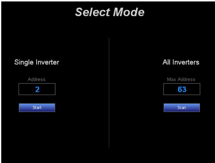
**Single Inverter:** insert the inverter address and the press Start
