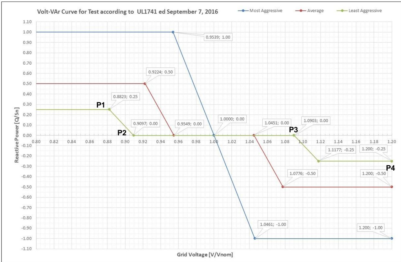
Figure 10: Volt-VAr Most (blue) and Least (grey) aggressive curves for ABB inverters
