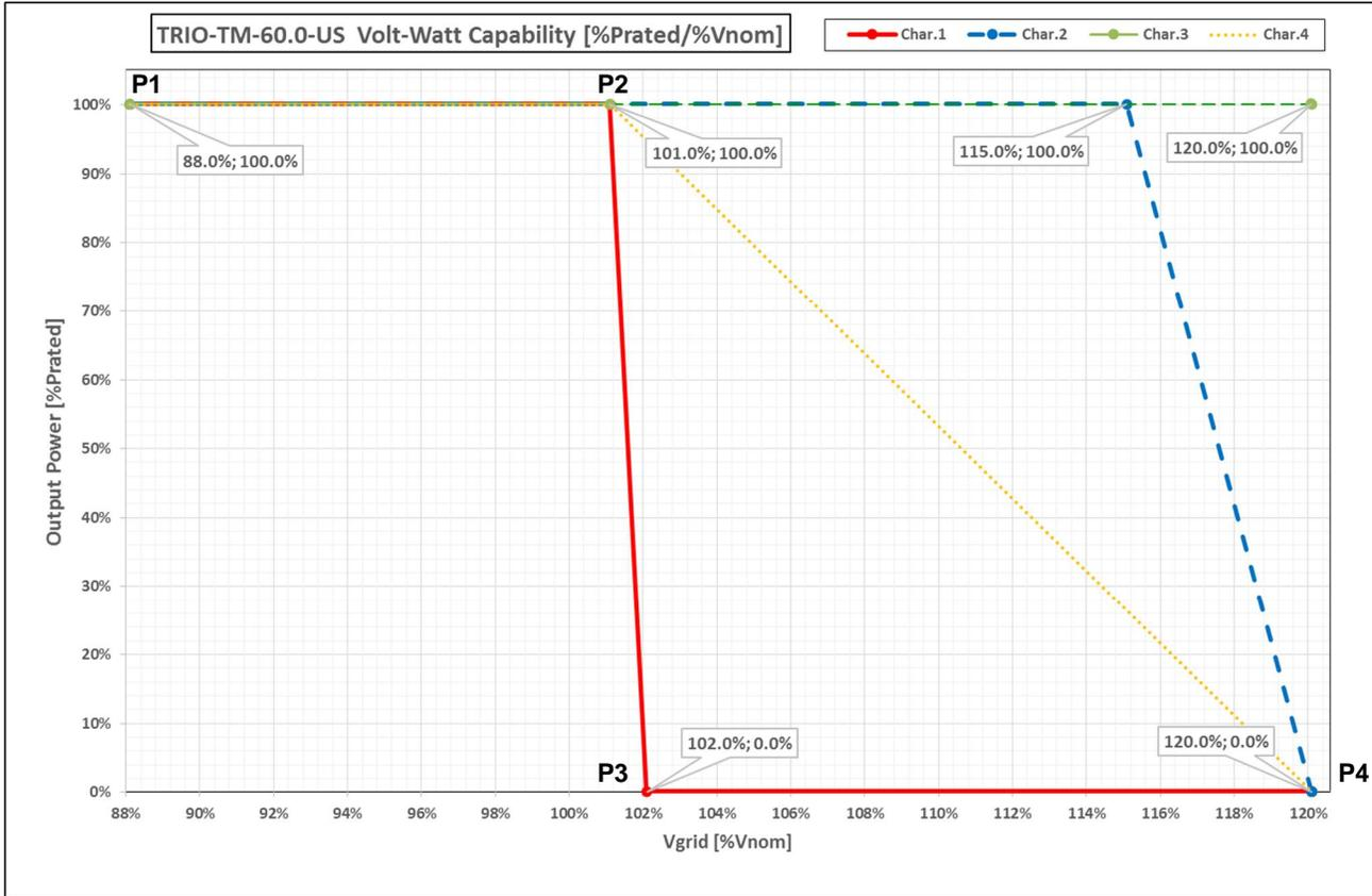
Figure 13: Test of Volt –Watt curve
