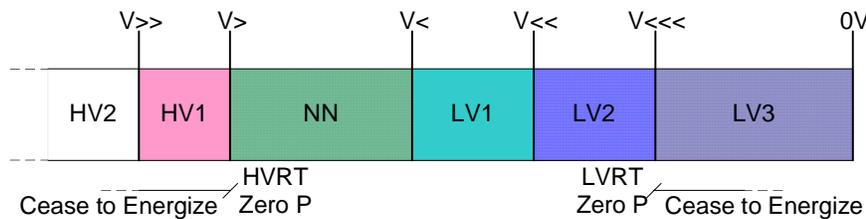
Figure 4: Inverter parameters and SA9 L/HVRT ranges
