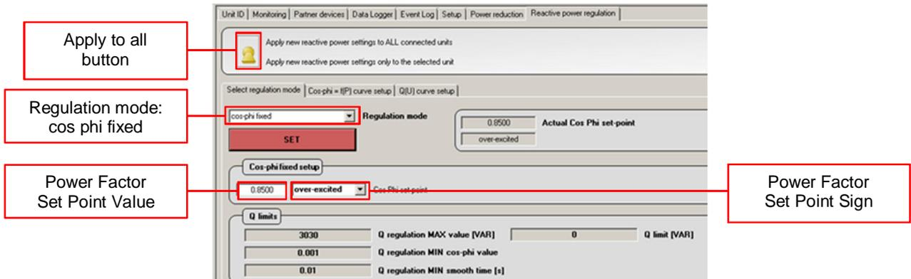
Figure 23: SA12 Specified Power Factor Configuration through Aurora Manager Lite
