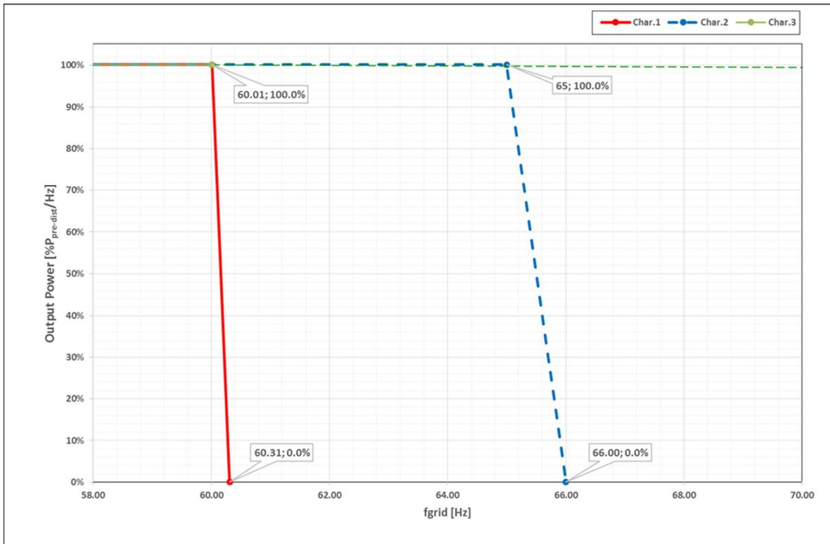
Figure 12: Frequency-Watt slope test
