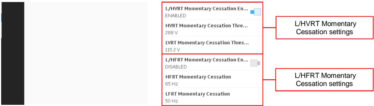
Figure 16: L/HVRT Configuration through Web Server
