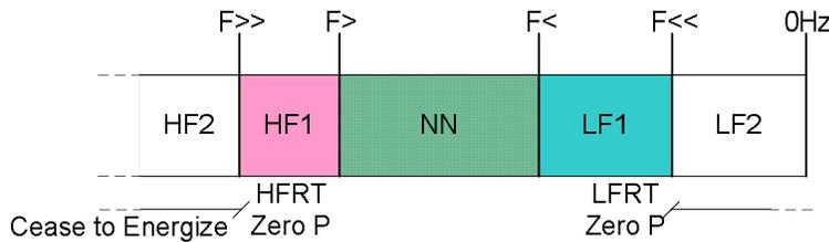
Figure 6: Inverter parameters and SA10 L/HFRT ranges
