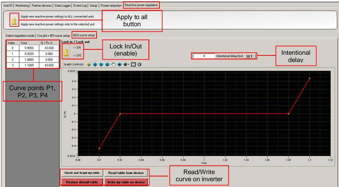
Figure 25: SA13 VV Curve Configuration through Aurora Manager Lite
