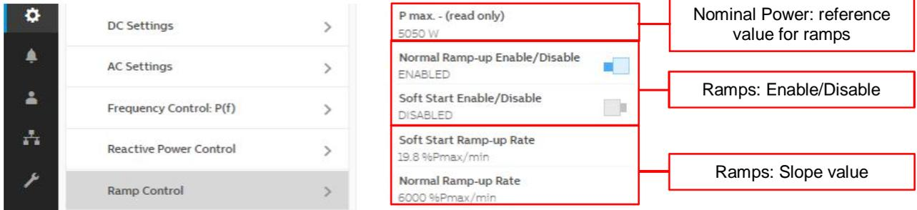
Figure 19: SA11 Normal Ramp Rate and Soft-Start Configuration through Web Server
