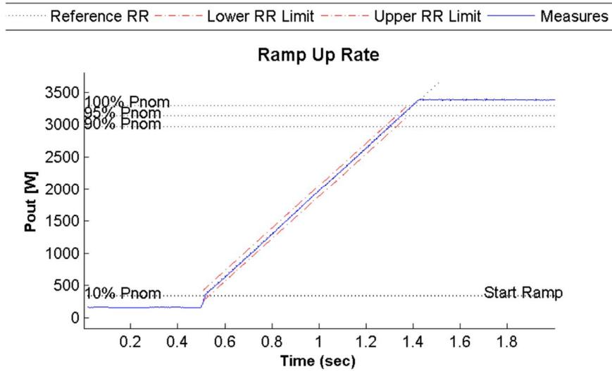
Figure 7: UNO-DM-PLUS-3.3, Normal Ramp Up @ 100% PN/s with upper and lower bound
