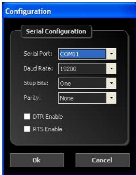
**Serial Port:** COM Port used to communicate with the inverters
