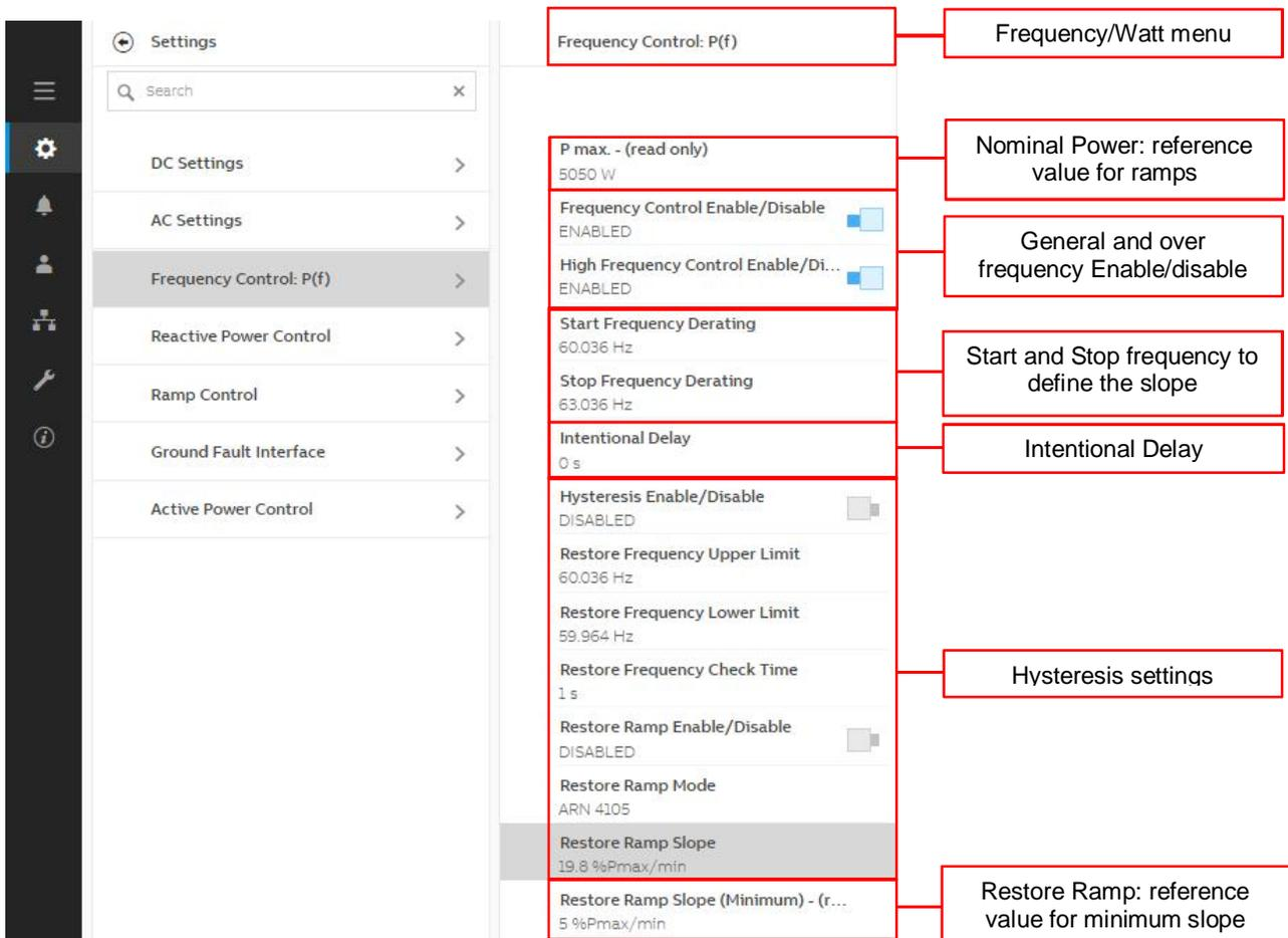
Figure 20: SA14 FW Configuration through Web Server
