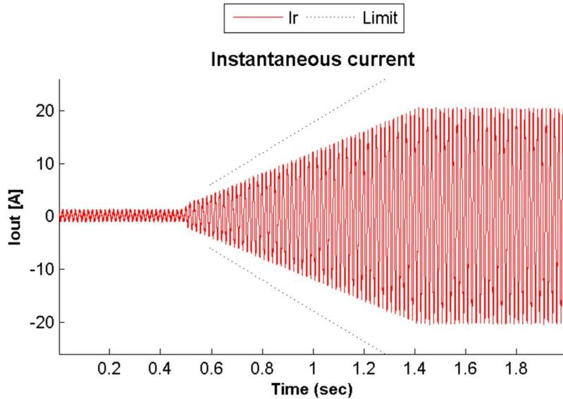
Figure 8: UNO-DM-PLUS-3.3, output current with upper and lower bound
