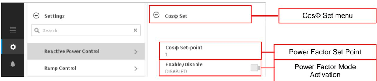
Figure 17: SA12 Specified Power Factor Configuration through Web Server
