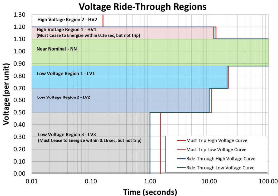
Figure 3: L/HVRT configuration example
