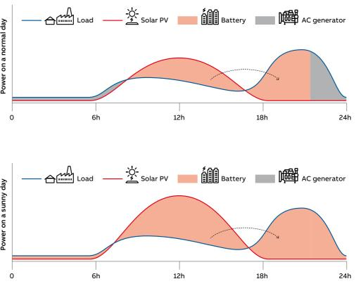
MGS100 prioritizes solar power during the day. After dark, the battery continues to supply power. If the battery runs out of energy, the AC generator (biofuel or diesel) will supply power for the rest of the night. Any excess energy produced throughout the day is used to charge the batteries. Once these are fully charged, excess energy can be sold to the grid to generate additional revenue.
