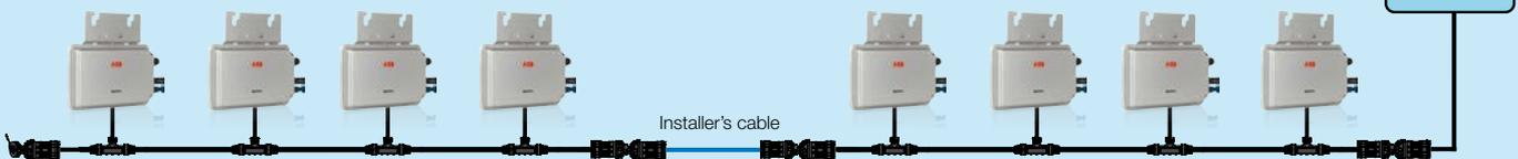
\* Always position the MALE CONNECTOR of the AC TRUNK BUS facing the junction box
