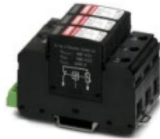
Surge arrester for 2-pos. isolated 1000 V DC voltage systems, for DIN rail mounting, 3-pos. base element with remote indication contact, three plug-in temperature-monitored protective elements, status message on each plug.
