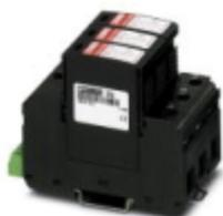
Universal varistor-based plug-in lightning/surge arrester for 3-phase power supply networks with common N and PE (4-conductor system: L1, L2, L3, PEN), with remote indication contact.
