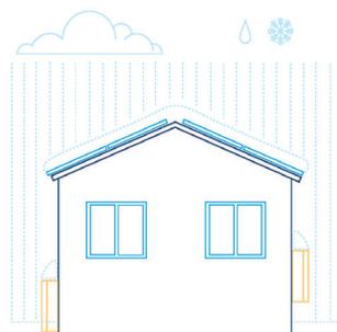
Air restricted by snow for both inverters - not properly installed
