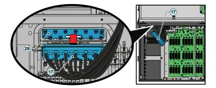
After the connection is made, the side screws on the AC/DC interface power connector (male) ((a) / (f)) have to be fasten with a tightening torque of 3 Nm. To check if the interface power connector (male) ((a) / (f)) is correctly installated it's possible to use the Multi-functional tool ((a) following the procedure below:
