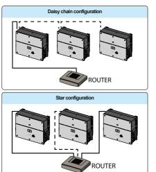
On each configuration of connection the maximum length of the cable must be 100m maximum between inverter - inverter and inverter - switch.
