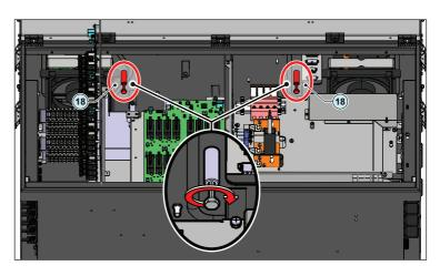
Close the positive string fuses plate (19) using the two M5 screws previously removed.
