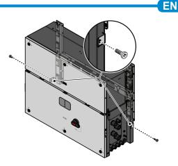
· Tighteen the two side screws (supplied) with a tightening torque of 5 Nm, to avoid the tilting of the bottom part of the inverter.
