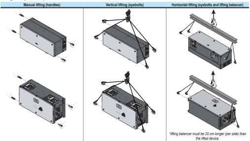
In case of manual lifting, for high height wall installation positions (>50cm floor distance from bottom side of the wiring box: this maximum allowed height value is calculated considering a medium tall height of 170 cm for operator) it's mandatory to use a support plan (e.g. a table) to place the equipment during the lifting operation, to allow the change of hands position. The use of the support plan is suggested also for <50cm height installation.
