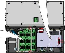
• Tighteen the two hexagonal junction screws (18) with a tightening torque of 12 Nm.
