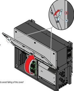
Open the cover and use the cover support brackets (1) to lock the cover in open position.
