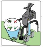
Connect the strings (refer to "Input connection to PV generator (DC side)" chapter) and check that the GREEN LED corresponding to each positive fuses activates. The string will turn out to be inverted if the green LED is OFF or, in some circumstances, faintly ON. It's recommended to check the strings one by one so to safely check wich strings are inverted.
