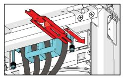
• Check if the fork of the Multi-functional tool (26) fit in the groove of screws of the interface power connector (male) (26) / (17): if it fits, the interface power connector (male) (26) / (7) is correctly assembled.
