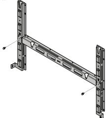
Use the two M8 screws with flat and spring washers (supplied) to fix the pieces of the bracket together.
