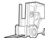
Powered industrial forklift (load-bearing capacity ≥ 4 t; recommended tyne dimensions: length ≥ 1800 mm, width 230–300 mm, thickness 25–80 mm)
