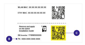
NOTE - The "Communication Identification Label" is located on the side of the inverter; this part of the label can be detached and placed in a more accessible location for later use, such as on the front cover of the quick installation guide.
