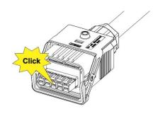
Insert the seal inside the connector body and screw the cable gland (6.5Nm)
