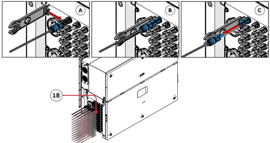
**NOTE** – It is highly recommended to put labels on each cable in order to easily reconnect them to the correct connectors once completed the service activities.
