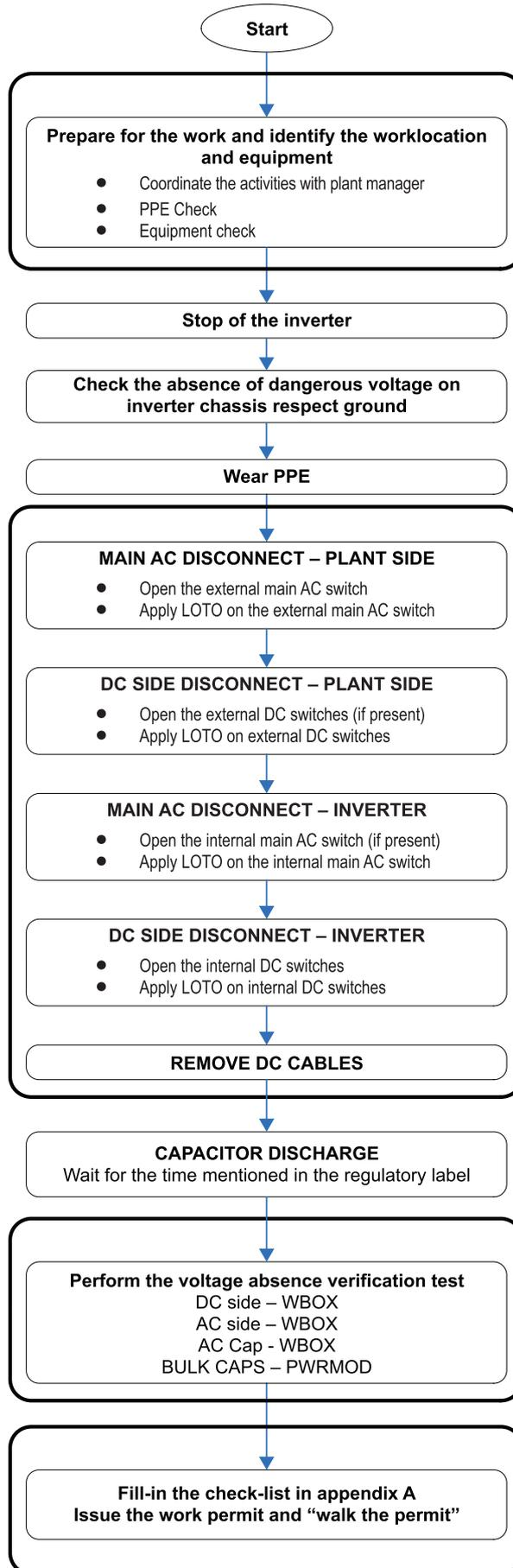
**⚠ WARNING** – Some inverter parts may be subject to hazardous voltages for the operator. Before performing any work on the inverter, follow this procedure for safely isolate the inverter.
