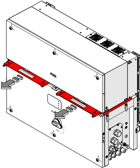
**NOTE** – Gasket protective covers and handles can be reused for a new installation.
