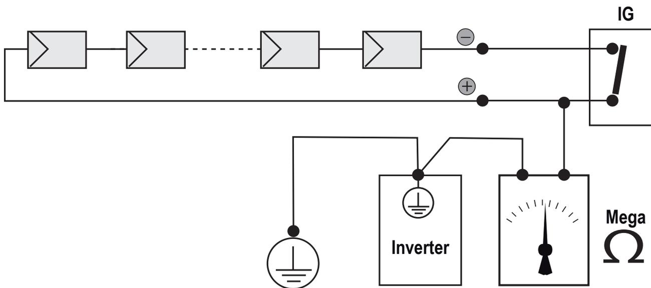
If the measured isolation resistance ( $R_{iso}$ ) is less than 75 kOhm, the inverter may not connect to the grid because of low isolation of the PV generator to ground.
