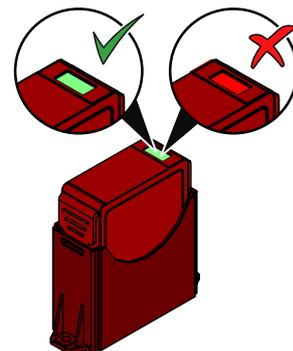
The DC surge arrester cartridges (24) are installed on the DC surge arrester plate (21) inside the wiring box (02).
