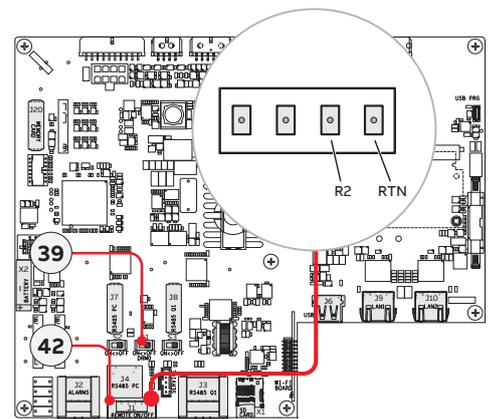
**NOTE** – In case of the DRM0 function is activated without the proper wiring of the Remote terminal block (42), the inverter will no longer be able to connect to the grid. For further information regarding the DRM0 function refer to the AS/NZS 4777 standard.
