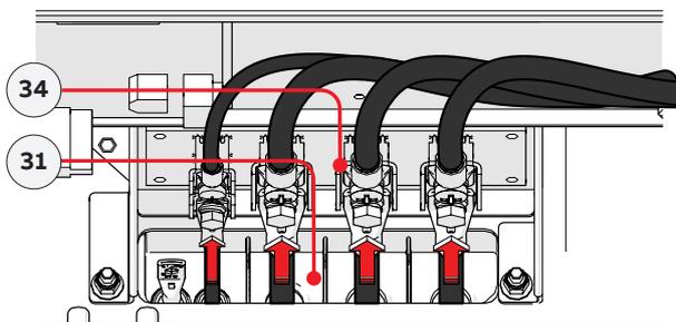
**⚠ ATTENTION** – In case of a wrong phase sequence the inverter will not connect to the grid and it will provide an error state.
