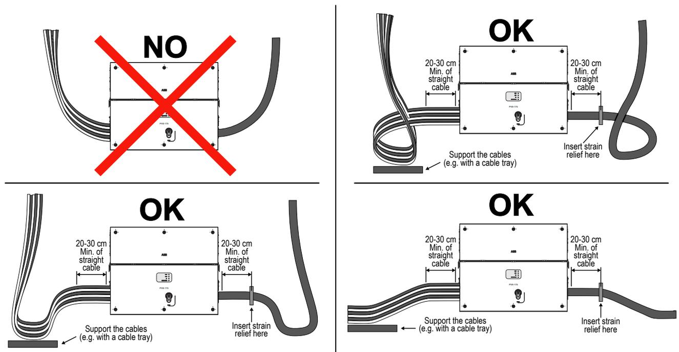
**⚠ ATTENTION** – In case of the AC cable glands (11) was accidentally removed during the cable routing phase, it will needed to assure the correct tightness of the lock nut of the cable gland to the inverter chassis with a tightening torque of 8.0 Nm (for each cable gland).
