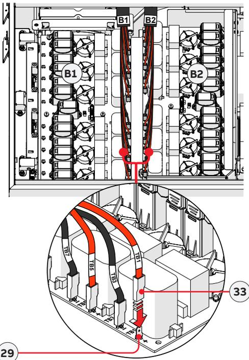
**⚠ WARNING – Polarity inversion can cause serious damage. Check polarity before connecting each cable!**
