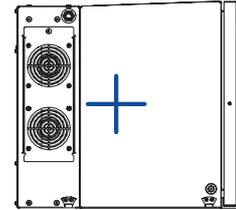
Center of gravity (wiring box)
