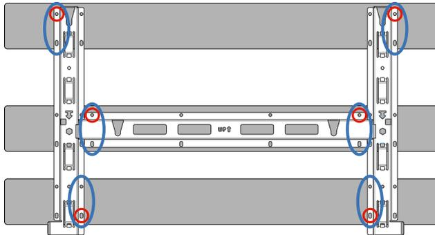
**Frame mounting (3 supports) minimum fixing points**
