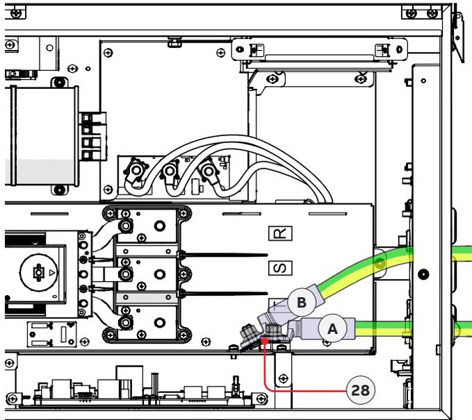
⚠ **ATTENTION** – Depending on the version of the AC panel installed on the inverter it will be necessary to use a different protection earth connection point in order to avoid mechanical stress due to cable bending: in case of Single-core AC panel use the horizontal connection point (A), otherwise in case of Multi-core AC panel it will be necessary to use the oblique connection point (B).
