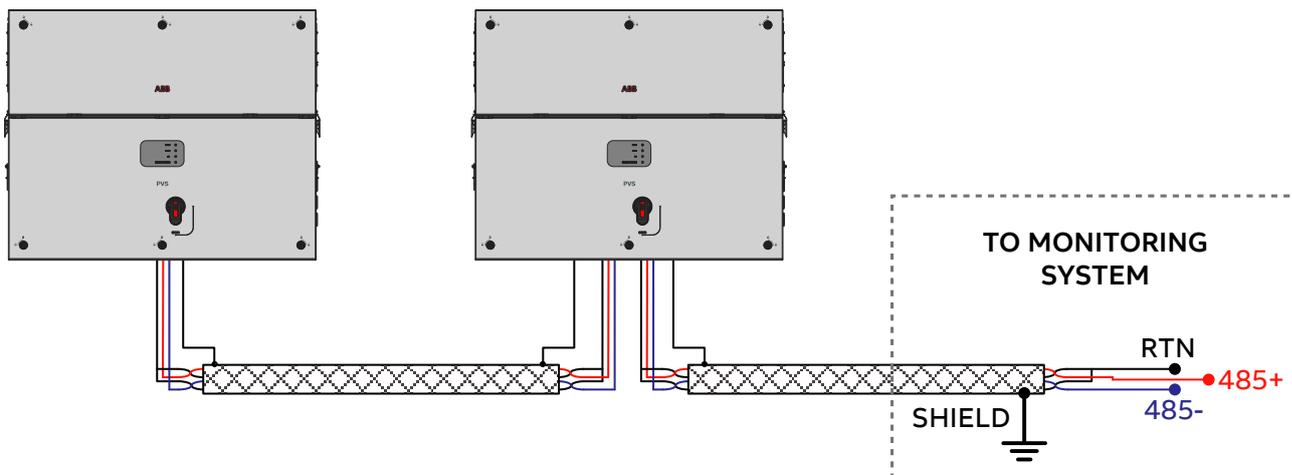
**NOTE** – It is the installer’s responsibility to evaluate the use of an additional overvoltage protective devices on the communication line.
