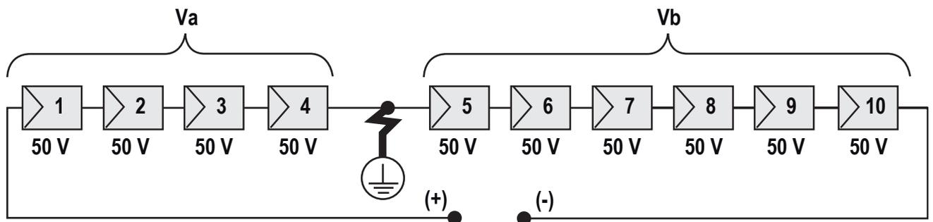
Va = voltage measured between + pole and  $\oplus$  = 200V
