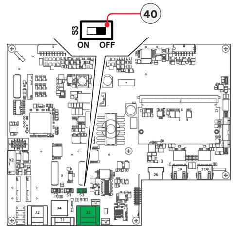
**NOTE** – Each inverter is shipped with the RS485 address pre-set to “2” and with the resistance terminal setting Switch **(40)** in the OFF position.
