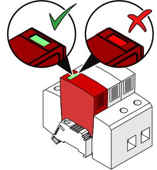
The AC surge arrester cartridges **(25)** are installed inside the wiring box **(02)**.
