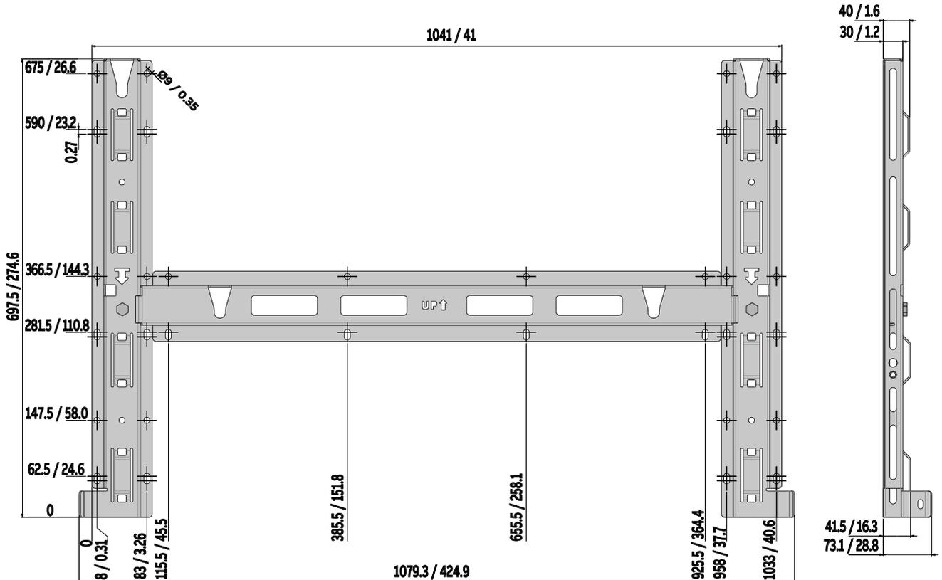
The diameter of holes in the bracket are 9mm / 0,35".
