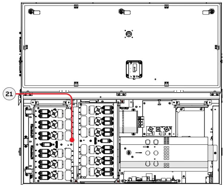
The layout of the DC surge arrester boards **(21)** is provided below, with reference of the points where the input DC voltage absence test must be performed. The points are represented by the faston where the cables (coming from DC switches **(19)**) are connected.
