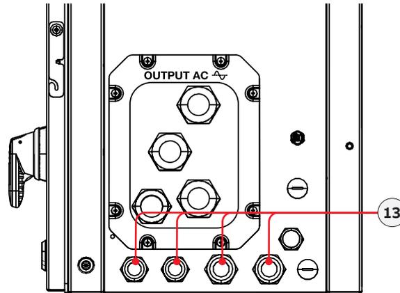
**⚠ ATTENTION** – The connection of the communication and control signal cables should be done with no over-length of the above mentioned cables. Moreover the communication and control signal connection cables should not be in contact with live parts.
