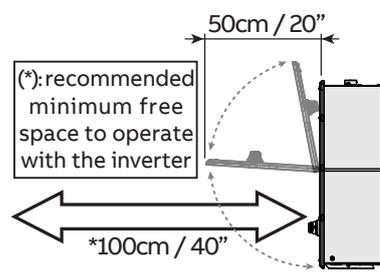
**⚠ ATTENTION** – Do not install any object (e.g. AC or DC cables) that could be damaged by overheating from outgoing hot air flow coming from top and side fan sections ( $\Delta T = +15\text{ }^{\circ}\text{C}$  compared to ambient temperature). In case of this kind of installation needs, please evaluate the installation of a proper air deflector. Always respect the minimum distances required.
