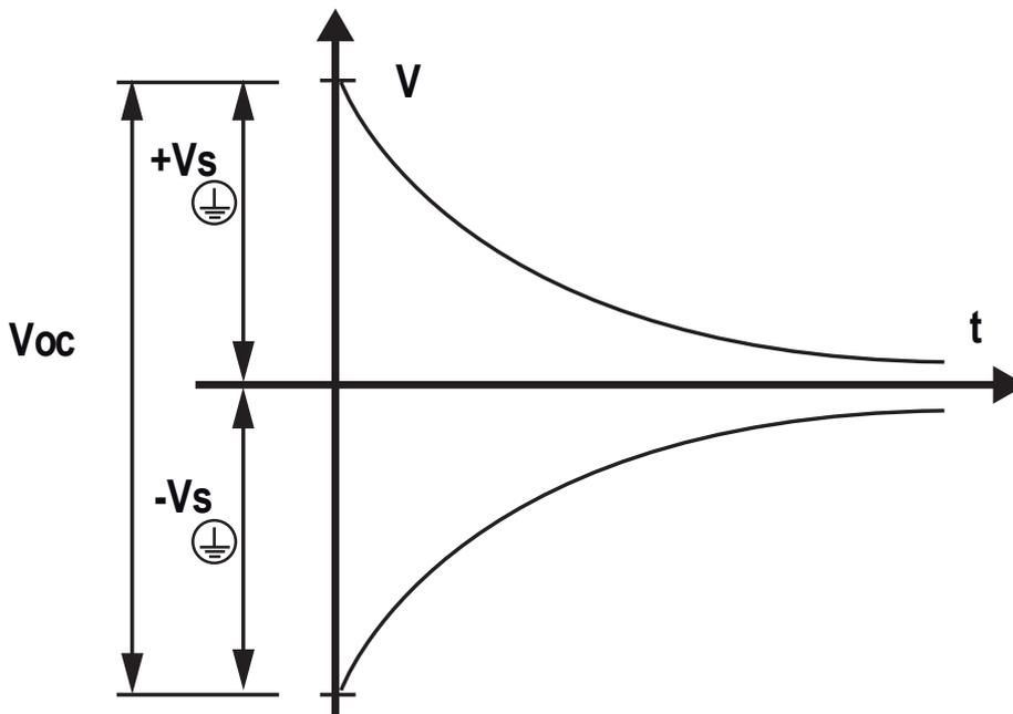
**NOTE** – The internal resistance of the voltmeter tends to zero the voltage present on the PV generator due to the capacitive effect.
