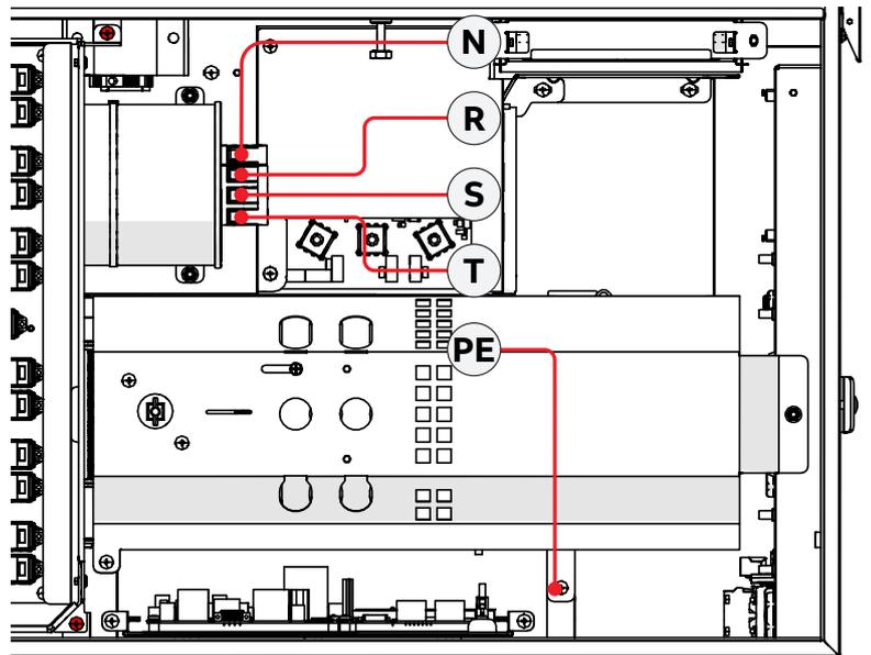
14. Voltage absence test on bulk capacitors (Power Module)
