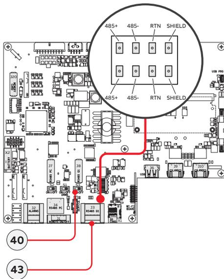
For long distance connections is necessary to use a shielded twisted pair cable with characteristic impedance of  $Z_0=120$  Ohm as shown on the following table:
