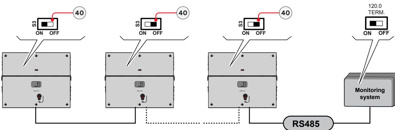
**NOTE** – The communication line must also be terminated on the first element of the chain which normally corresponds to the monitoring device.
