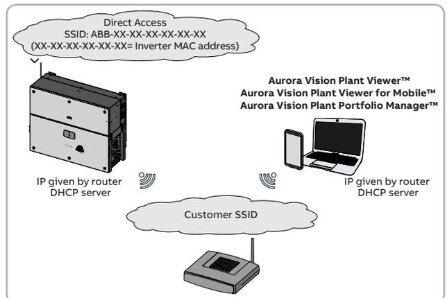
In case of connection to channel 2 (“Station Mode”), it will be required to enter the wireless network parameters (set on the router) and follow the subsequent procedure:
