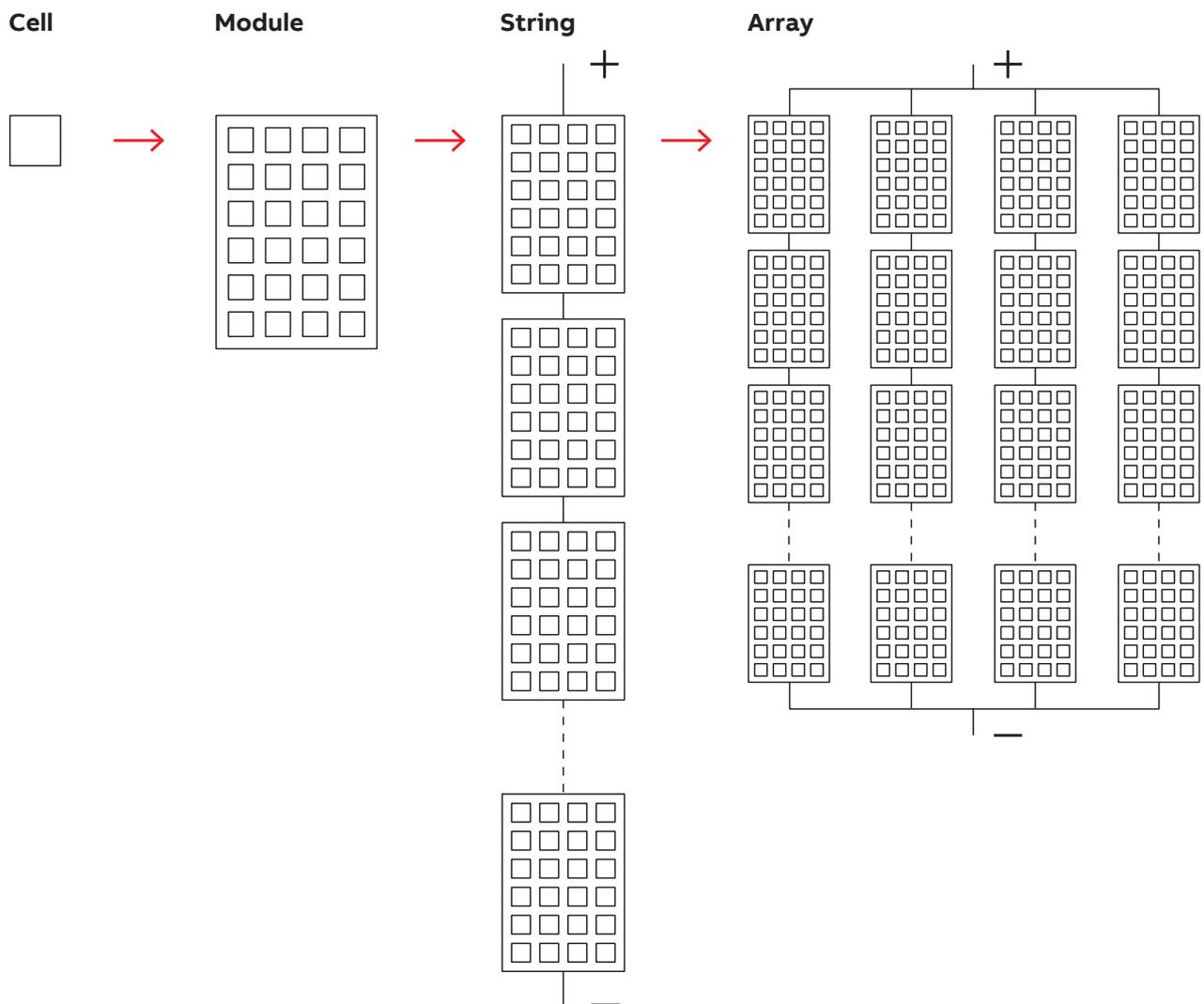
**ATTENTION** – The current of each array must fall within the rating value limits of the inverter.
