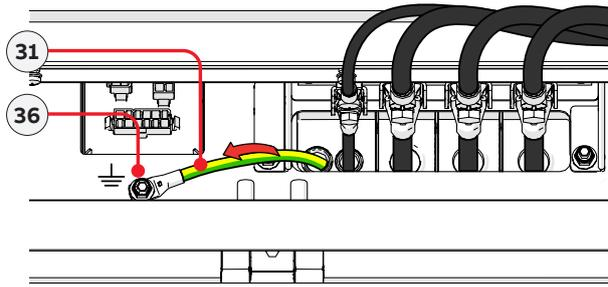
Use the washers and bolt supplied in the power module installation kit:
