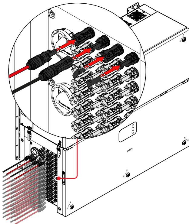
**⚠ ATTENTION** – If any string inputs is not required check that protective caps are installed to the relative unused connectors. This is necessary for the inverter seal and to avoid any damage to the unused connectors which may be used at a later time.
