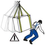
*During handling, do not make any sudden or fast movements that can create dangerous swinging.*
