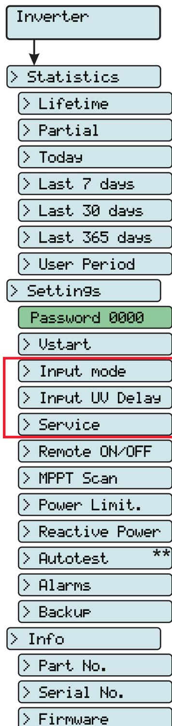
We advise changing the activation voltage only if really necessary and to set it to the correct value: the photovoltaic generator sizing tool available on the ABB website will indicate whether  $V_{start}$  needs changing and what value to set it to.
