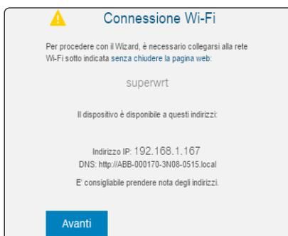
Once the REACT is associated with the domestic Wi-Fi network, the user must reconnect the tablet/smartphone/PC to the same Wi-Fi network as the REACT system. The key remains locked until this connection is established.
