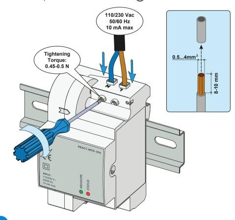
The REACT-MTR-1PH is equipped with an RS485 line that allows communication with the REACT system to maximise the system's self-sufficiency and self-consumption.
