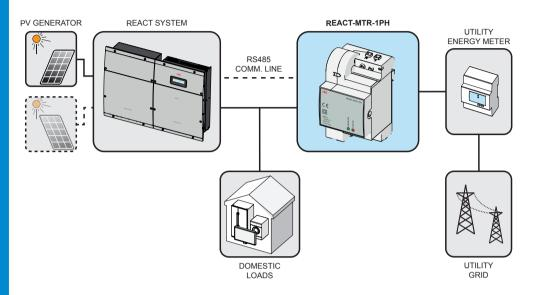
The REACT-MTR-1PH has two multicoloured LEDs, "Status" and "Measure", which show the status of the device and the direction of the energy flow (import / export of energy) in real time.
