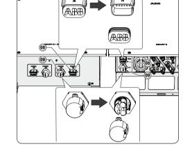
Connect the two battery cables between inverter and battery unit (supplied inside the REACT2-UNO box)
