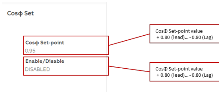
Figure 3: SA12 Specified Power Factor Configuration through Web Server
