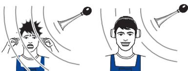
In the installation, consider or make sure the **noise emitted based on the environment** is not such that it exceeds thresholds allowed by law (less than 80 dBA).
