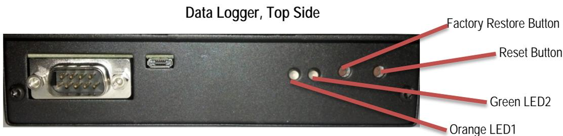
Checking the status LEDs on the logger is the first thing to do when troubleshooting a logger. A solid orange LED1 (or no LEDs lit with 24VDC present) is an indication that the logger is not running properly and may need replacement if the problem persists.
