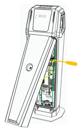
5. Since the front door is no longer fastened to the station, it can be removed completely.
