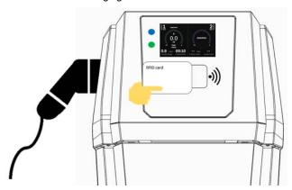
13. The LED will turn a steady GREEN color. When the display shows a message indicating that you should remove the cord from the socket being used, please do so
