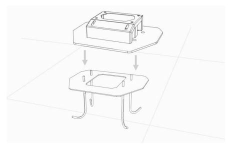
3. Fasten the stand to the plate with clamps using M10 bolts and M10 washers (available in the clamp base package) to be screwed onto the protruding threaded parts with a tightening torque of 36-46 Nm.
