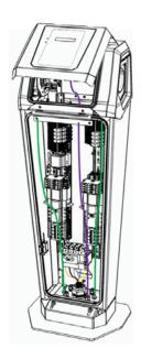
3. Close the cover and re-tighten the two M5 screws and their washers previously removed with a tightening torque of 4.3-5.5 Nm.
