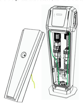
6.Remove the main disconnect switch's terminal covers and remove the two drain hoses from the 2 metal hose adaptors.
