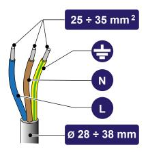
The following table shows the maximum length of the conductors in relation to the chosen section:
