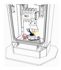
3. Reattach the two drain hoses to the 2 metal hose adaptors.
