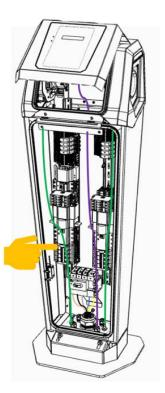
2. Verify the correct connection (L1-L2-L3-N-PE) making sure that the respective positions of the phases and neutral in the main disconnect switch are correct, as well as verifying that the ground protection is correctly connected to its dedicated terminal.
