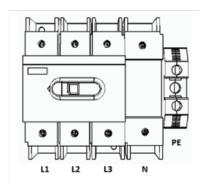
3. Place the disconnect switch terminal covers on the lower terminals (previously removed).
