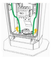
7. Using a ratchet for hexagonal screws, unscrew the 4 fixing bolts and their washers from the bottom of the station, separating the stand and the plate from the station with cord glands (CAUTION: as indicated in step 2, be sure to place the station on a horizontal plane before removing the hexagonal screws to avoid dropping the station body when removing the screws)
