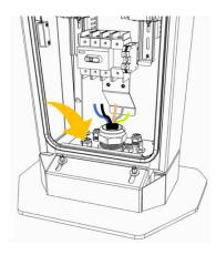
2. Reuse the Ø10 hex head screws and Ø10 washers (previously removed during unpacking) to secure the plate with cords gland to the bottom of the station (and consequently the station to its stand) with a tightening torque of 36-46 Nm.
