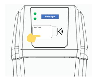
7. The station opens the available socket (or both if free). The user must insert the charging cord within 50 seconds, ensuring that the cord is fully seated in the socket
