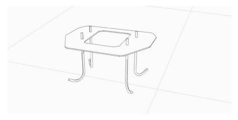
2. Once the concrete solidified, place the stand on top of the upper part of the plate with clamps, so that the protruding threaded parts pass through the holes in the stand, and run the corrugated cord through the stand.
