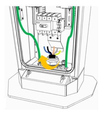
2. Strip the wires to a length of 18-21 mm for the power supply cable and neutral wires, and 17 mm for the ground cord. Connect the ground cord to the respective terminal and tighten with a torque of 3 Nm and then connect the phases and neutral to the main disconnect switch (after removing the terminal covers), making sure that the entire ferrule of each cord is fully threaded (the tightening torque for the terminals of the disconnect switch is 6 Nm).
