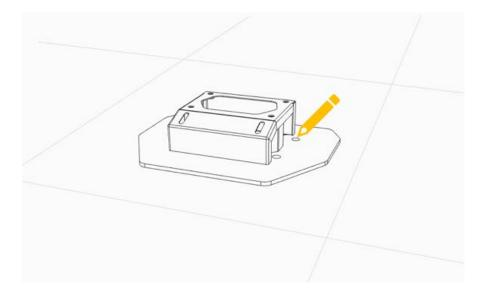
3. Remove the stand and drill holes in the ground at the position of the 4 marks previously made with a 12 mm drill bit to position the anchoring devices. The maximum drilling depth is 60 mm for at least 120 mm thick soils, and 80 mm for at least 160 mm thick soils. Then, clean the hole made from any debris of drilling.
