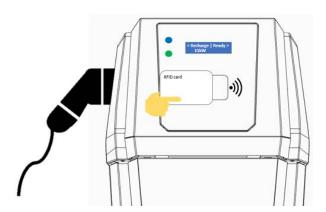
2. The LED will turn a steady GREEN color. When the display shows a message indicating that you should remove the cord from the socket being used, please do so
