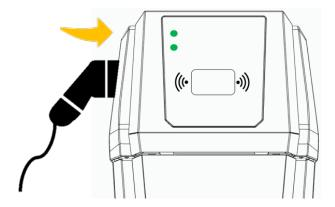
4. Charging starts and the LED corresponding to the socket used turns steady BLU
