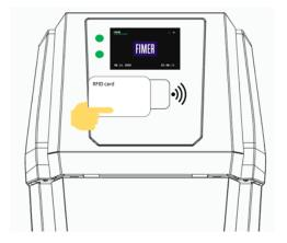
5. The station opens the available socket (or both if free). The user must insert the charging cord within 50 seconds, ensuring that the cord is fully seated in the socket
