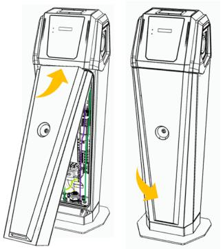
6. The last operation is to lock the door using the special key. It is advisable to keep the door against the station casing until the lock has been closed.
