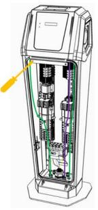
2. Plug the available end of the Ethernet cord into the lower right side of the station's head, where an Ethernet port is available.
