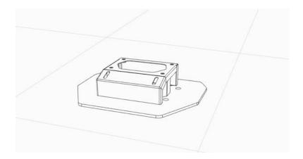
2. Using the stand as a template, make marks on the floor at the position of the 4 present holes.
